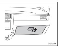
Open the glove box by pulling the bottom of the handle upward. Close the glove box with a firm push.
